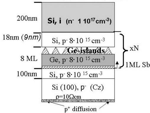
Schematic structure of a Si/Ge QD solar cell with layers of Ge quantum dots in the active layer of the Si solar cell substrate
