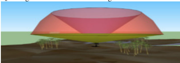
Scanned volume(using multiple elevation angles)
