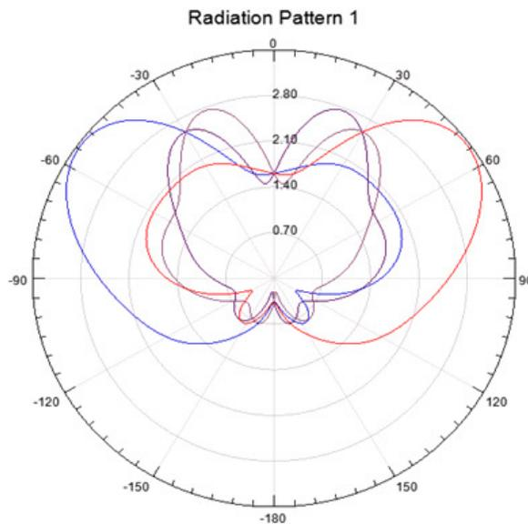
Figure 4: Broadside Radiation Pattern of Simulated Radiating Patch
