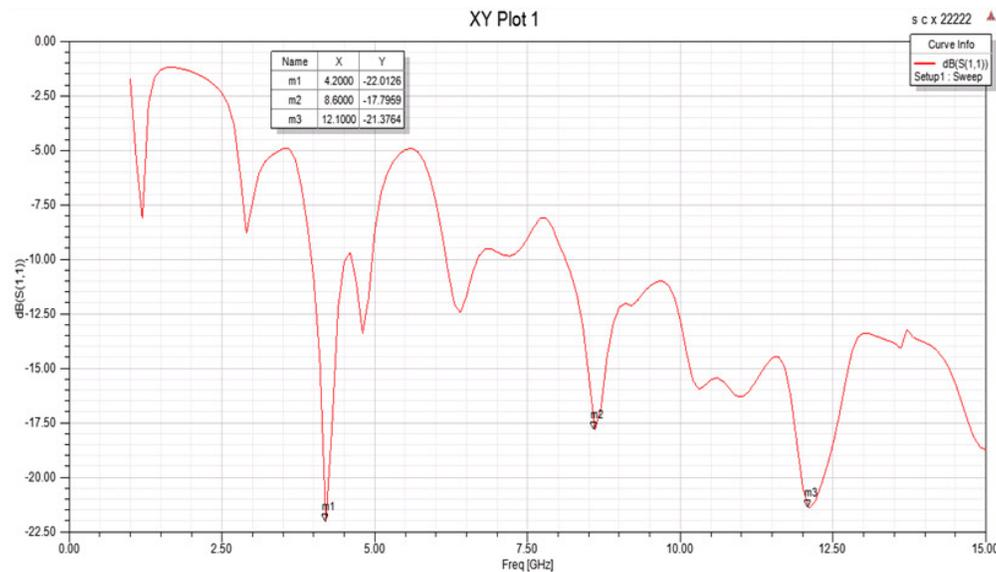
Figure 2: Return Loss Parameters of the Simulated Antenna
