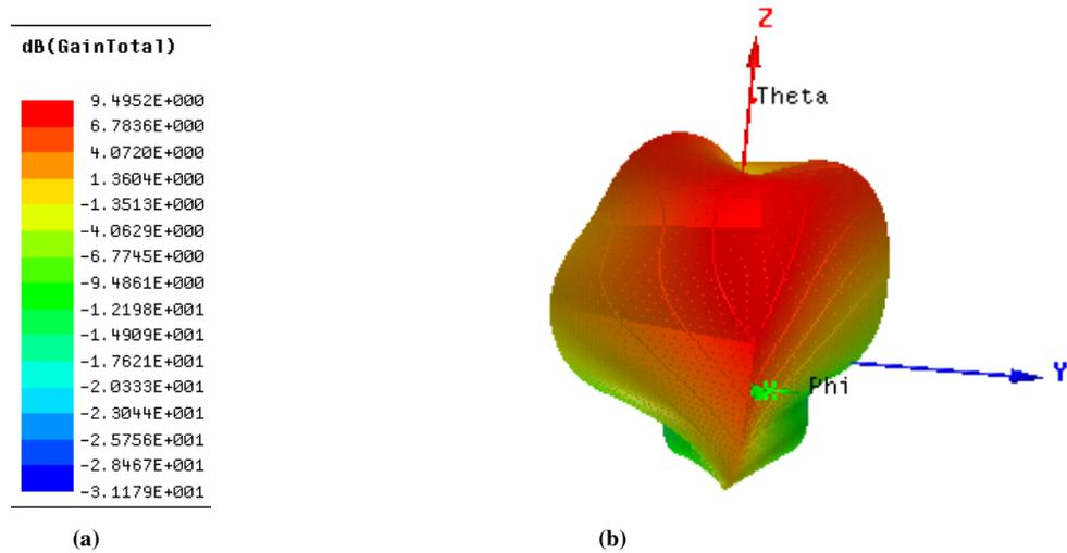
Figure 3: (a) Gain Value for the Slot Simulated Slot Antenna ; (b) 3 D Plot of the Gain realised
