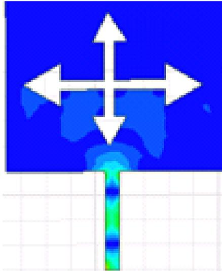
Figure 1: Current Distribution Diagram for the Proposed UWB Antenna.
