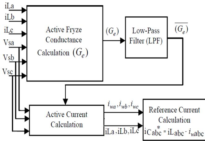
Fig. 5 Block diagram of FPT method
