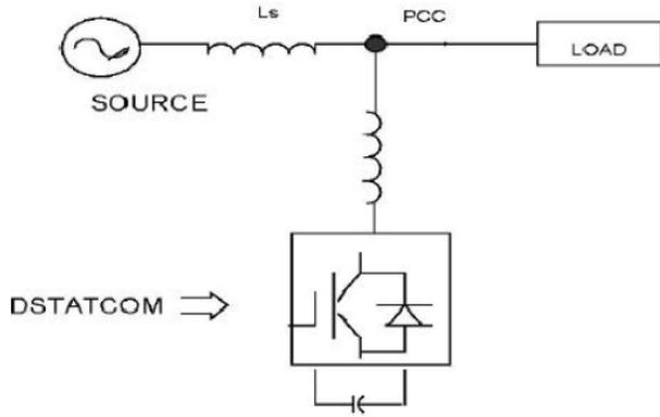
**Fig. 3 Block Diagram of DSTATCOM**
