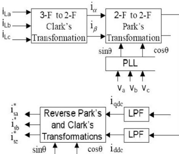
Fig. 6 Block Diagram of SRFT
