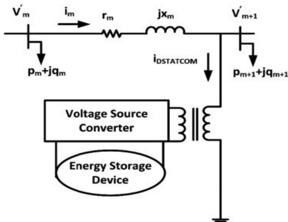
Fig. 1 Operating Principle of DSTATCOM
