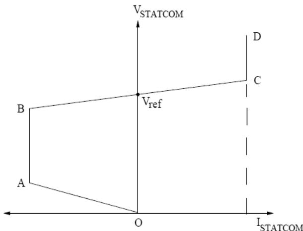
**FIG. 4 Operating Characteristic of DSTATCOM**
