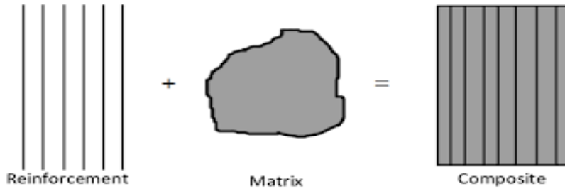
Fig 1.0 scheme of reaction between matrix and reinforcement
