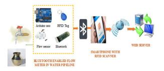
Fig. 1 Architecture of Smart Water Management
