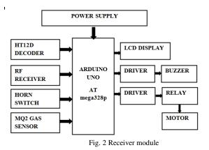
The schematic diagram as shown in Fig 2 consistof Arduino UNO, HT12D Decoder, RF Receiver, MQ2 Gas Sensor, 12v DC motor and Relay Contactor. The Arduino has various features for communicating with a computer, another Arduino, or other microcontrollers[10]. It provides serial communication. The data is received(RF Receiver) from the RF transmitter. The RF receiver consists of four pins [7].
