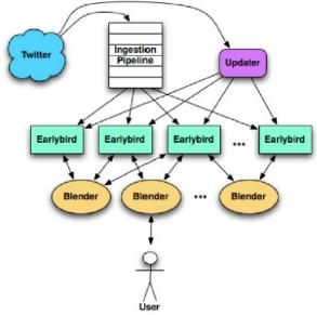
Fig. 1 Architecture of Earlybird-Twitter's real-time search engine
