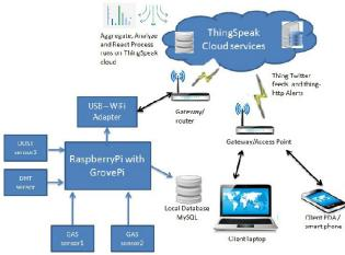
Fig 3.1: Overall system architecture
