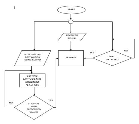
Fig:6-Flow diagram of Receiver Section
