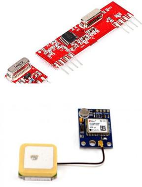
MEA format which is the most common format used by all GPS receivers. The requirement of power for this GPS module is very low.
