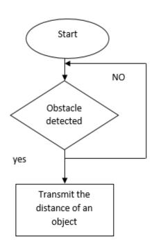
Fig:5-Flow diagram of Transmitter Section.
