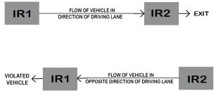
Fig. 1 Initialization of sensor to find the vehicle violating the rules.
