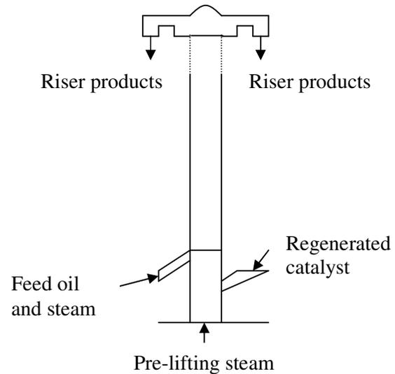
Figure 2: The FCC riser reactor
