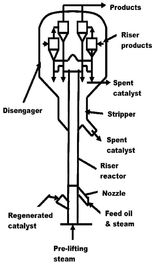
Figure 1: The FCC reactor
