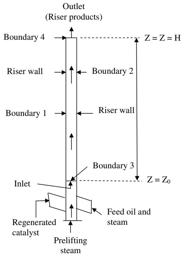
Figure 3: The FCC riser reactor without termination device simulated
