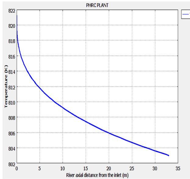
Figure 4: The temperature in the riser reactor
