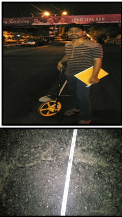
Fig -2: Ravelling Measurement, Rutting Measurement
