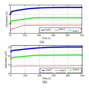
Fig. 12. Real-time measurements of first-harmonic impedance measurement for different loads during heating (a) equivalent resistance R1 and (b) equivalent inductance L1.
