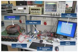
Fig. 10. Experimental prototype
