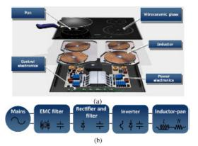
Fig. 1. Domestic induction cooktop: (a) exploded view and (b) general block diagram.
