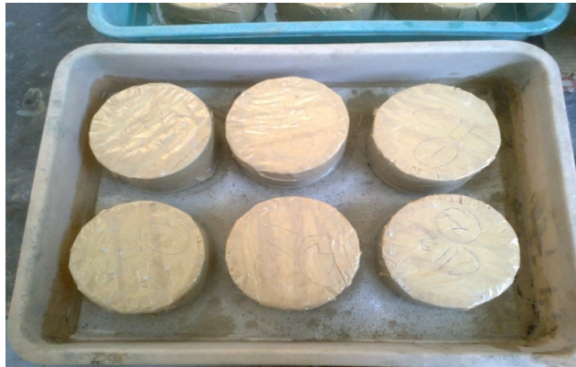
Fig. 3.5 Sorptivity test setup
