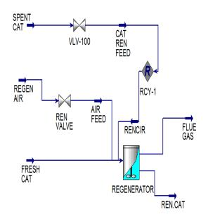
Figure 3: Model and simulated diagram of FCC Unit Regenerator.
