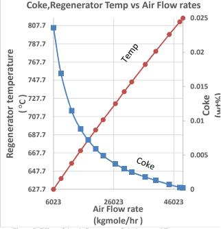
Figure 7: Effect of the air flow rate on Coke burnt and Temperature.
