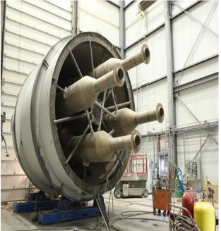
Figure 2: Regenerator cyclone separators
