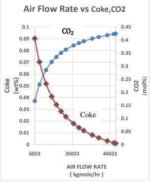
Figure 6: Effect of the air flow rate on the Coke burnt and CO<sub>2</sub> mole fraction.
