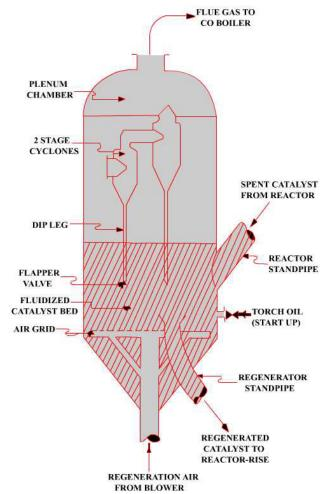
Figure 1: Schematic of FCCU Regenerator
