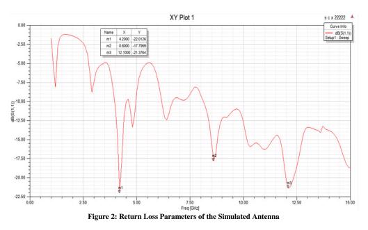
The return characterics have been realised as shown in Figure 2. The required return loss characterics have been realised in the frequency bands of 4.2GHz, 8.5GHz and 12.1 GHz, as -22.01dB, -17.79dB, -21.37dB respectively. The said antenna is designed on FR4 substrate, with a dielectric constant of 4.6/ The microstrip antenna layout
