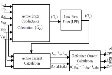
Fig. 5 Block diagram of FPT method
