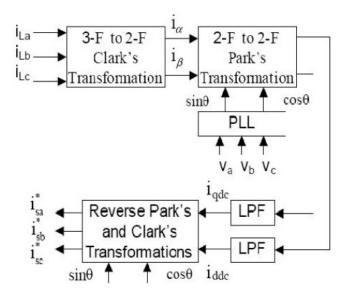
Fig. 6 Block Diagram of SRFT
