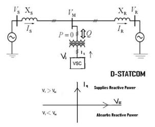
Fig. 2 The single line diagram of DSTATCOM
