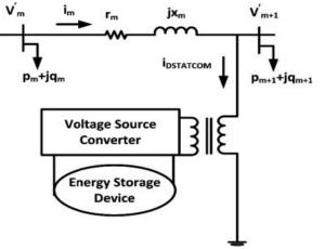
Fig. 1 Operating Principle of DSTATCOM
