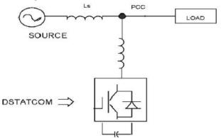
Fig. 3 Block Diagram of DSTATCOM
