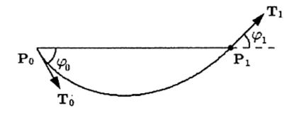
Figure 1 initial condition schematic diagram Cubic Bézier curve can be expressed:
